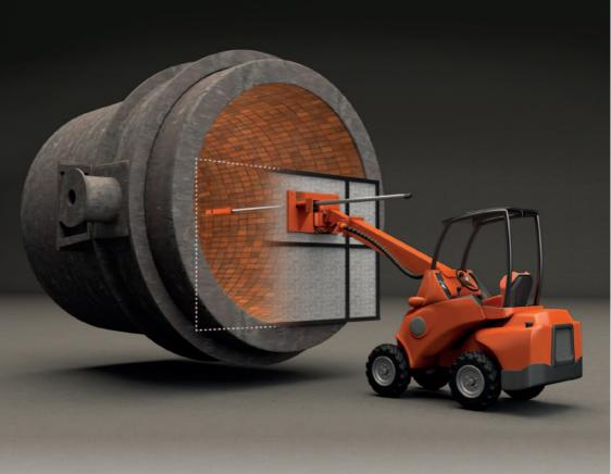
Reveal 360 is the complete solution for monitoring inner surfaces of ladles, converters, furnaces at high temperature condition. A lance with its sensor kit (laser, camera) is introduced inside the target and quickly collects data from the whole surface by rotating at 360 degree angle in a few steps.
